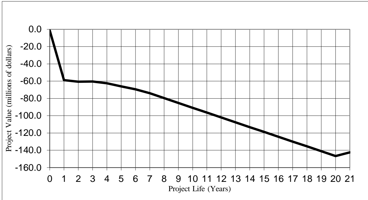
Figure 2.1. Cumulative non-discounted cash flow diagram for the anhydrous ammonia process. A project life of 20 years, construction period of one year, taxation rate of 35%, and a MACRS 5-year depreciation schedule was assumed.
